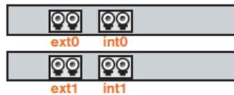
The network path to be protected is connected to any two like-numbered interfaces. The “ext” interface always faces an external Internet connection, and the “int” interface always faces the internal network, as shown in Figure 1-2: Inline mode Deployment. Do not send outbound traffic from the internal network to an “ext” interface. Pravail treats all traffic on “ext” interfaces as external.
