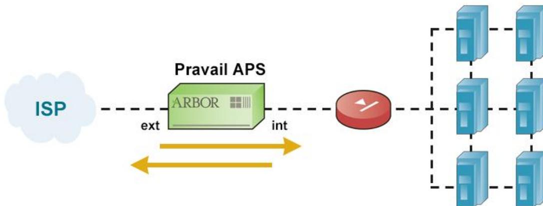
An additional option that Pravail APS supports is Cloud Signaling. Cloud Signaling is the process of requesting and receiving cloud-based mitigation of volumetric attacks in real time from an upstream service provider. In short, if the Pravail APS determines that thresholds for rate-based attacks are met, the TOE will signal the ISP or MSSP (via trusted channel) and the ISP or MSSP then mitigates the attack
