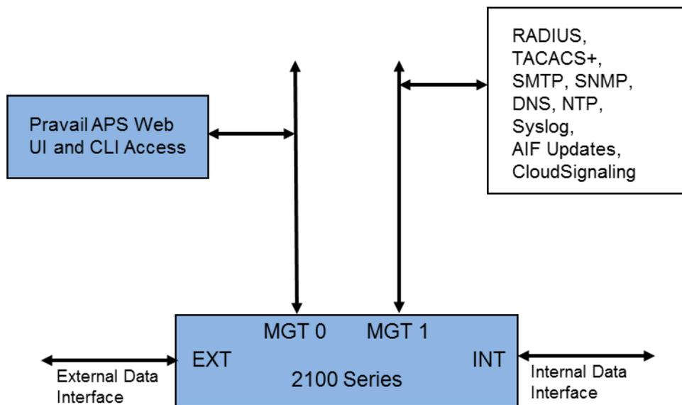
**Figure 1-5: TOE Physical Boundary (Blue components)**
