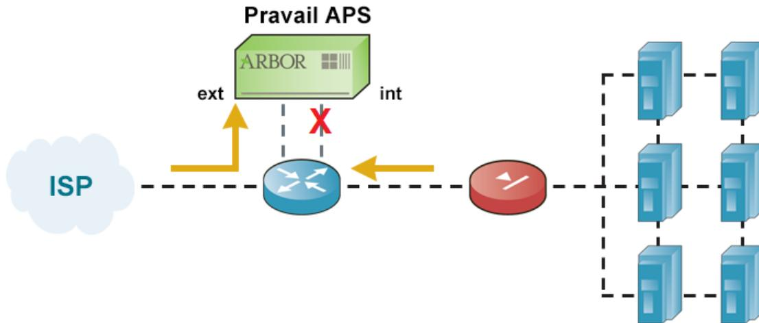
Pravail APS inline mode can be operated in an “inactive” protection mode, in which it analyzes traffic and detects attacks without performing mitigations. The resulting information can be used to set/customize the APS policies for attack detection and mitigation. When the APS policy is ready for operational implementation, the administrator can change the protection mode to “active” and allow the APS to mitigate attacks.
